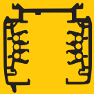
S-TRACK 3-phase system
